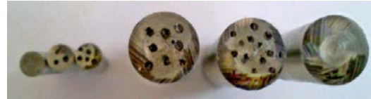
Fig. 8: Photographic view of ECM surface textured and non-textured A356 alloy pins
